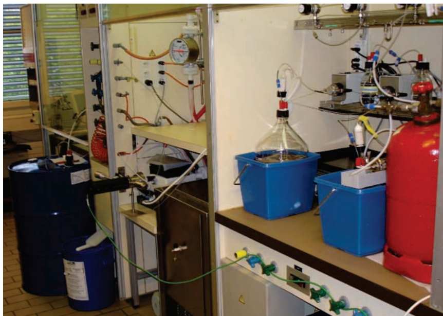
Figure 7. Kilogram-laboratory setup showing that the handling of solvent is now the bottleneck under intensified reactor conditions.
